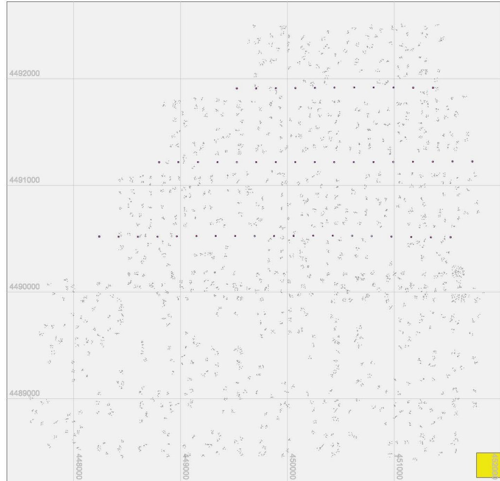
Graphic with 47 photos from the project. The camera locations are shown with its standard deviations for XYZ. The area has a planimetric extent of about: 4677 x 4510 [m].
