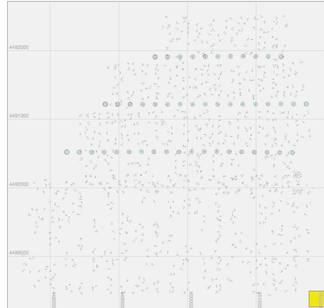
Graphic with 47 photos from the project. The camera locations are shown with its standard deviations for omega,phi,kappa. The area has a planimetric extent of about: 4677 x 4510 [m].
