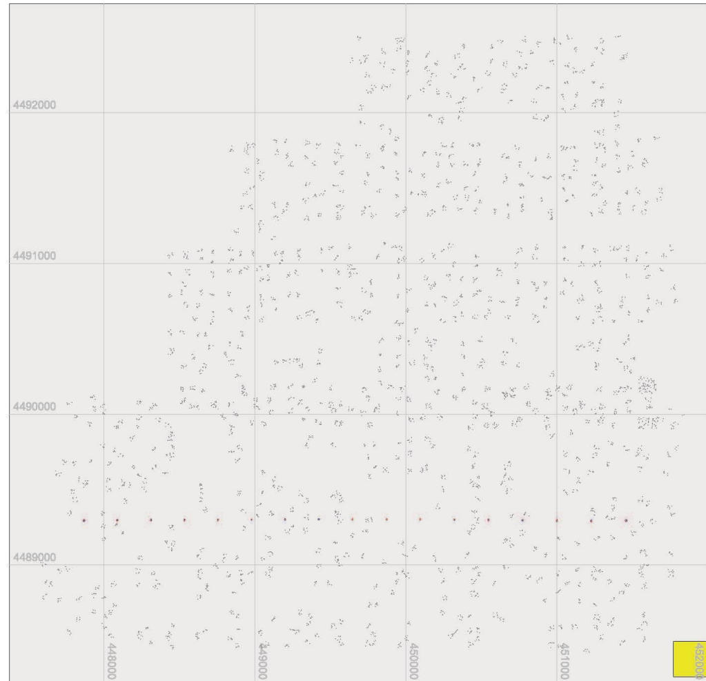
Graphic with 17 photos from the project. The camera locations are shown with its standard deviations for XYZ. The area has a planimetric extent of about: 4677 x 4510 [m].
